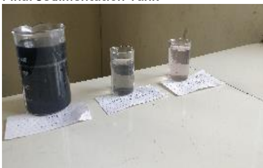
Wastewater at various stages of CETP
